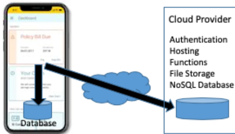
Figure 1: Local and Cloud Data Storage
