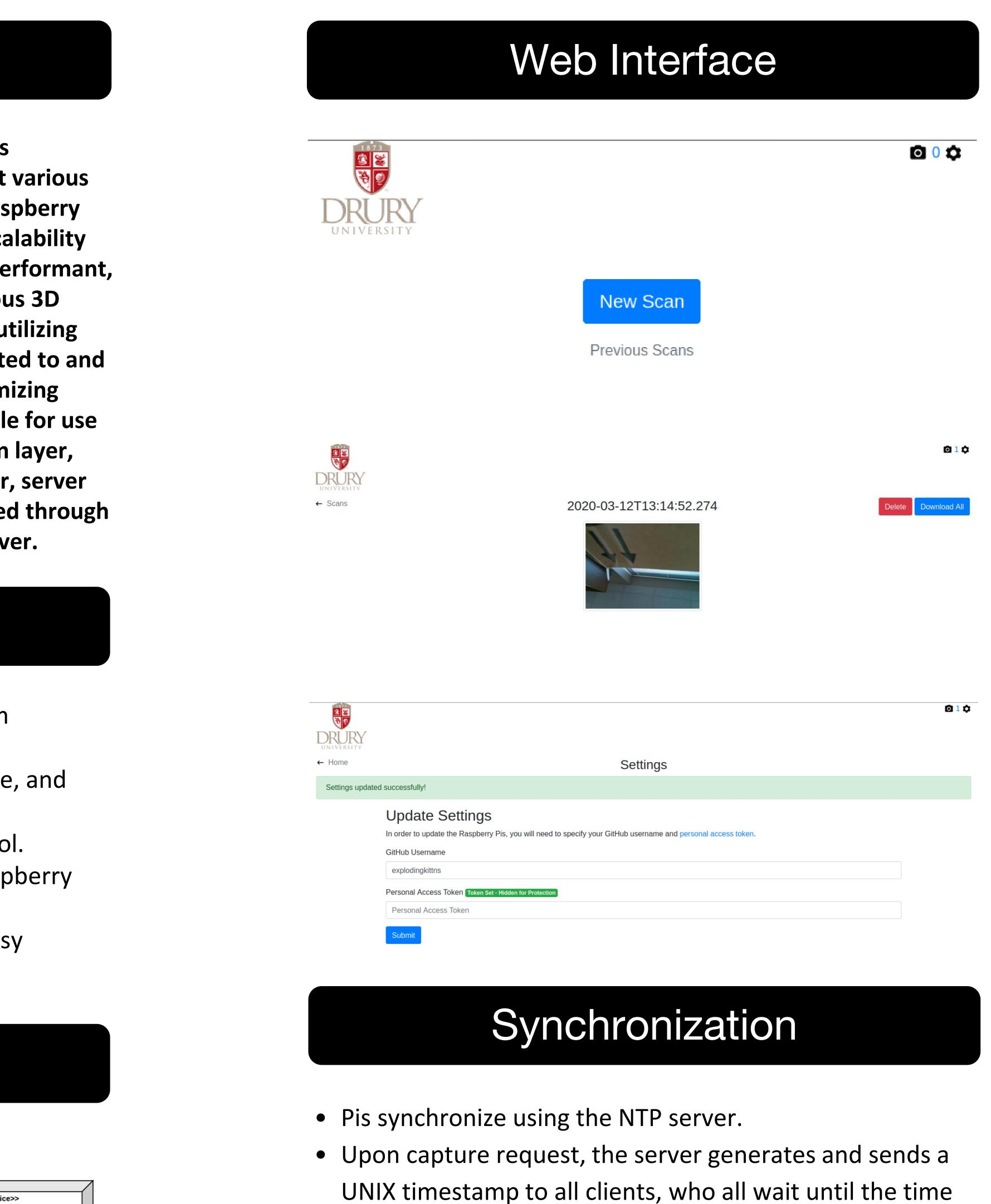
Decentralizing the waiting process allows for ~5 ms accuracy, regardless of the number of Pis.
