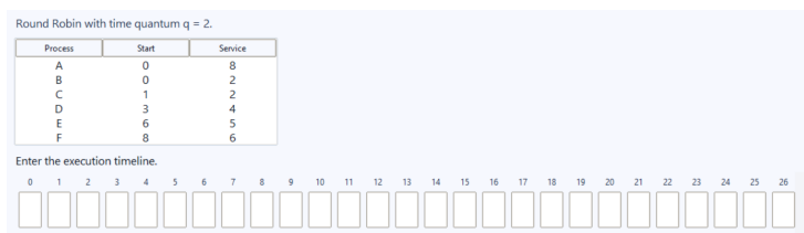
Figure 1: Round robin problem with a time quanta of 2.
