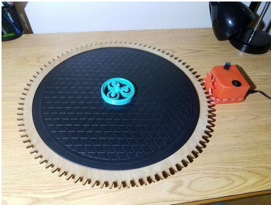
Figure 7: Turntable showing laser-cut wood gear and 3-D printed motor housing and gear.
