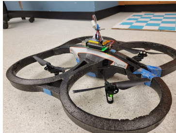
Figure 4: Raspberry Pi 3 atop Parrot AR 2.0 drone
